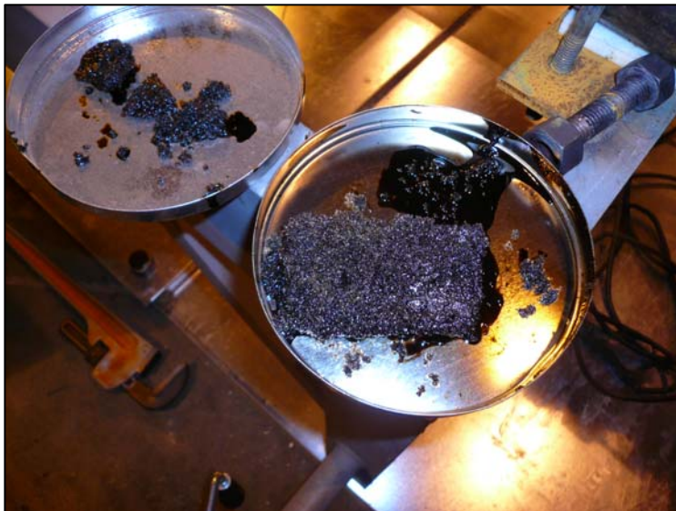
Figure 6. Hard Ice Scraped from Flow Loop
