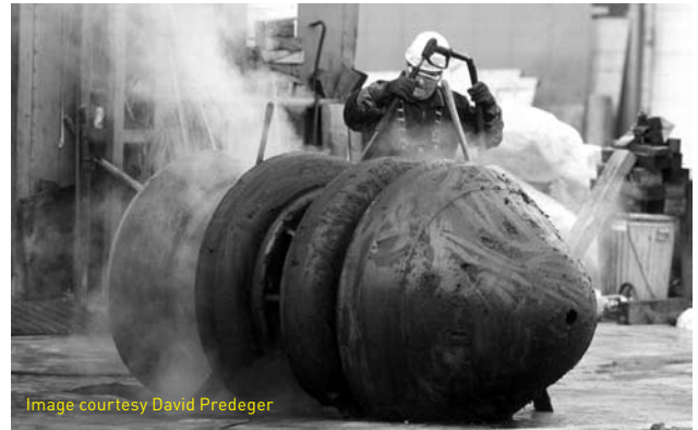
Image courtesy David Predeger TAPS employee cleans a scraper pig at the Valdez Marine Terminal. Scraper pigs, which clean the pipeline and enhance oil flow, are pushed by the oil.
